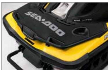
Reboarding platform with storage
