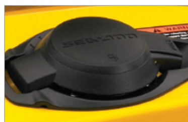
Quick latch fuel filler design
